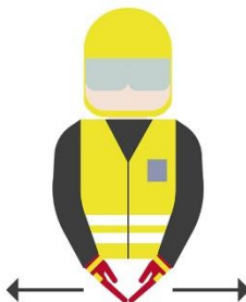
OPEN THE CRANE'S GRAB
