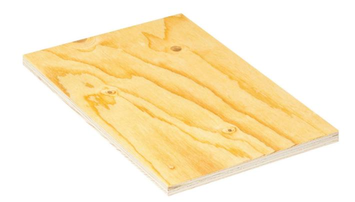
Metsä Wood Spruce FireResist is a surface impregnated softwood plywood with enhanced fire performance. The European reaction to fire classification for Spruce FireResist is B (according to EN 13501-1). The product is suitable for interior applications, and it must be protected from weather exposure at all times. The product is suitable for internal and protected external use in humid conditions. Panel must be protected from weather exposure at all times.
